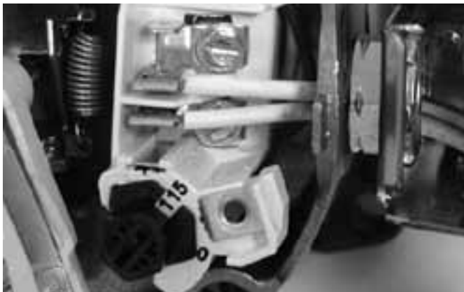
Figure 7: Voltage set to 115 volts, Dial Type
